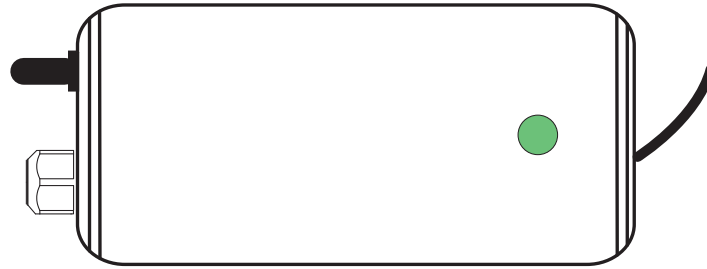
Green LED indicates UV lamp “ON”.
